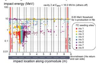
Figure 3: Impact energy versus impact location along the cryomodule. Emitters start in cavity 2 ( $E_{acc} = 16 \text{ MV/m}$  for cavity 2, zero for all others) distinguishing between iris 1 through iris 8 (see color code in legend).
