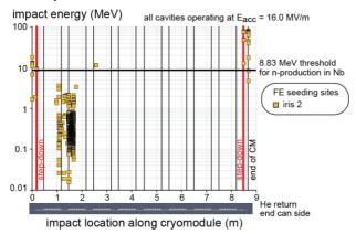
Figure 4: Impact energy versus impact location along the CM. Emitters start in cavity 2 at iris 2 ( $E_{acc} = 16 \text{ MV/m}$ ).
