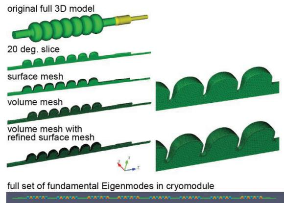
Figure 1: Top left: Modeling and FEA meshing sequence by means of a bare JLab upgrade cavity. Top right: Corresponding close-ups of the mesh. Bottom: Electric field contours of all accelerating modes in the full CM.
