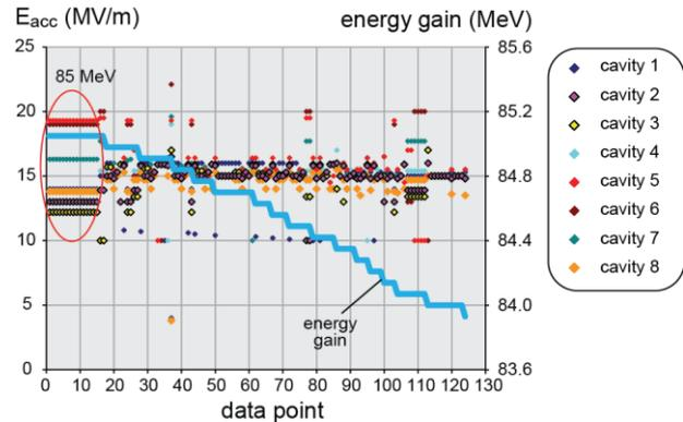
Figure 6: Field levels in individual cavities during radiation surveys (covering a full month) with C100-1 delivering an energy gain (blue line) of 83.9-85 MeV.
