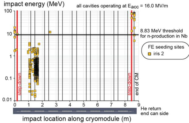
Figure 4: Impact energy versus impact location along the CM. Emitters start in cavity 2 at iris 2 ( $E_{acc} = 16$  MV/m).
