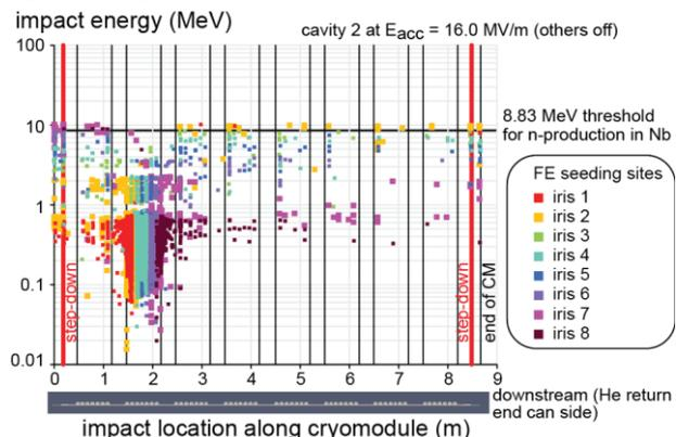
Figure 3: Impact energy versus impact location along the cryomodule. Emitters start in cavity 2 ( $E_{acc} = 16$  MV/m for cavity 2, zero for all others) distinguishing between iris 1 through iris 8 (see color code in legend).
