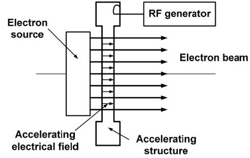
Fig. 4: Physical concept of an electron accelerator with wide beam using a toroidal cavity
