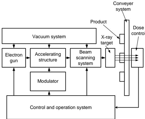
Fig. 1: General structure of an industrial irradiator based on a linear electron accelerator.
