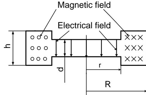
Fig. 5: Distribution of electrical and magnetic field in a toroidal cavity.
