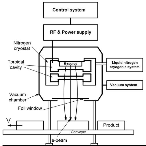
Fig. 11: Electron accelerator for radiation technologies with electron source inside cavity, two toroidal RF accelerating structures, and no magnetic focusing.
