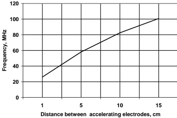
Fig. 6: The dependence of toroidal cavity frequency on the distance between accelerating electrodes for  $r = 50\text{cm}$ ,  $R = 100\text{cm}$ ,  $h = 40\text{ cm}$ .
