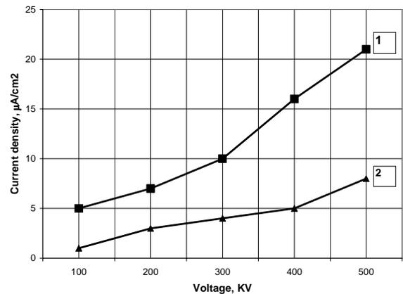
Fig. 8: Carbon fiber cathode emission characteristics for cathode and anode separations of 5 cm (1) and 10 cm (2).
