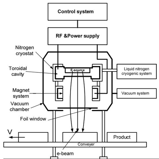
Fig. 10: Electron accelerator for radiation technologies with electron source inside of the RF cavity.
