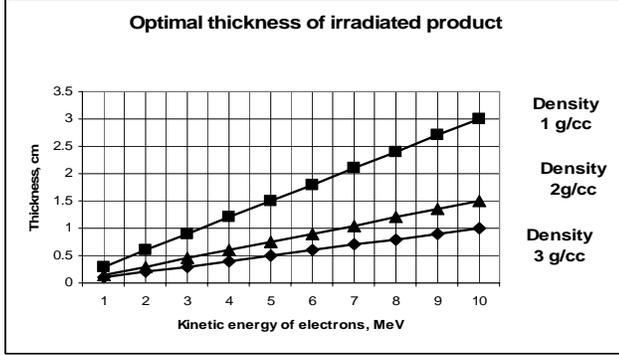
Fig. 3: The optimum thickness of a product irradiated by an electron beam as a function of electron beam energy for three different densities.
