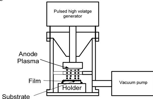
Fig. 12: Pulsed high voltage ion/electron film deposition.
