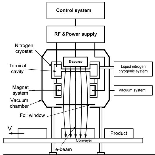
Fig. 9: Electron accelerator for radiation technologies with the electron source outside of the RF cavity.
