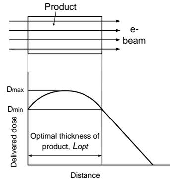
Fig. 2: The distribution of delivered dose from electron beam irradiation from one side.
