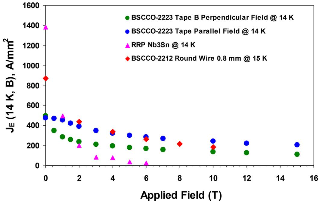
**FIGURE 14.**  $J_E$  comparison at 14 -15 K between Nb<sub>3</sub>Sn, BSCCO-2212 wire and BSCCO-2223 tape as a function of applied magnetic field.
