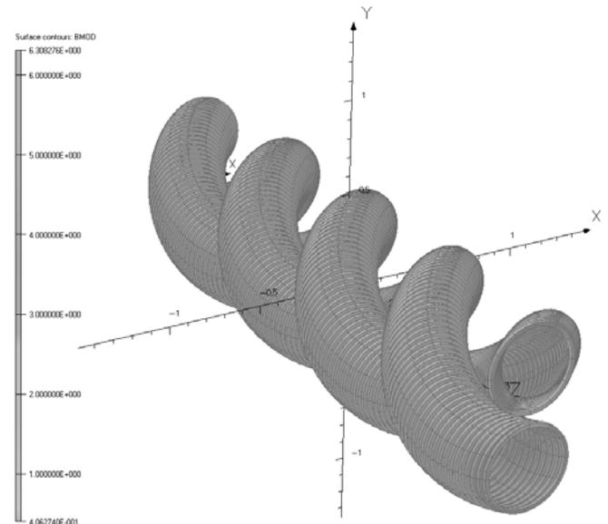
Fig. 4. Double Helical Solenoid geometry and flux density.
