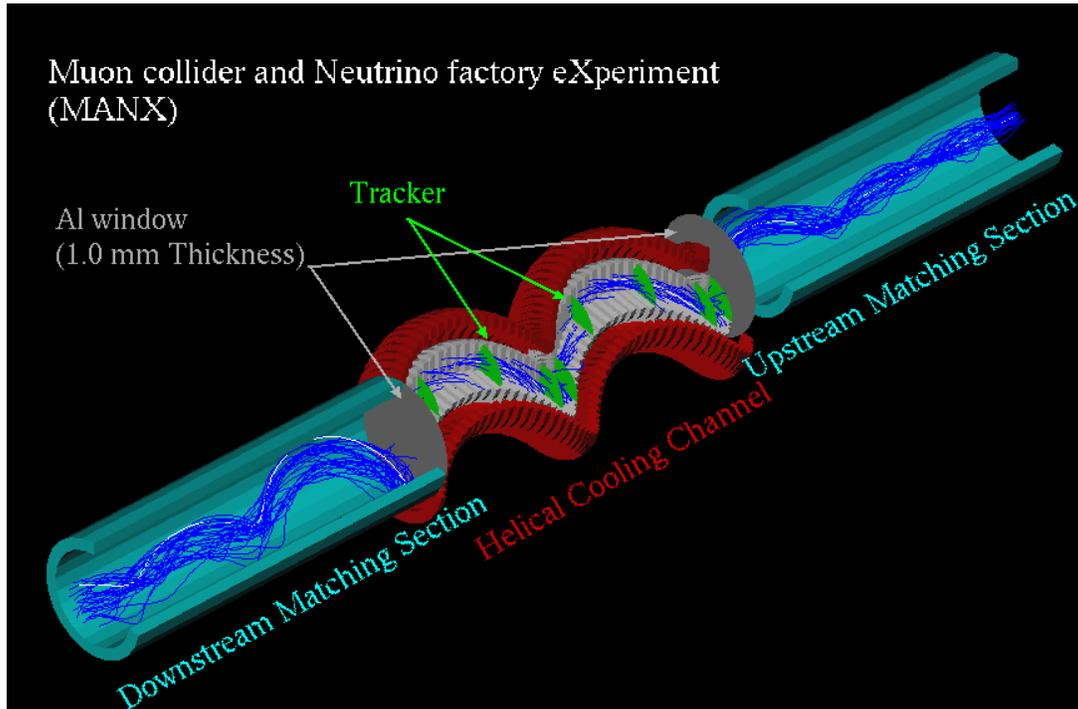
Figure 9: Conceptual picture of the MANX apparatus. The helical solenoidal magnets shown in red enclose the LHe ionization energy absorber, which is separated from the vacuum of the matching sections by thin Al windows.
