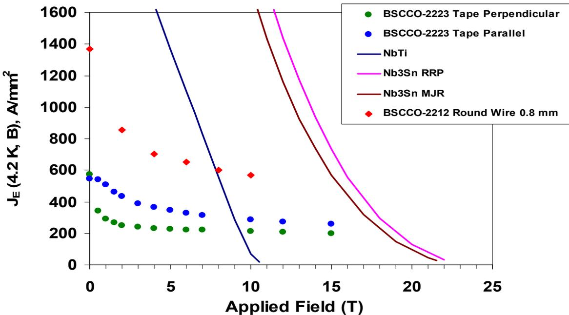
FIGURE 13.  $J_E$  comparison at 4.2 K between NbTi, Nb<sub>3</sub>Sn, BSCCO-2212 wire and BSCCO-2223 tape as a function of applied magnetic field.
