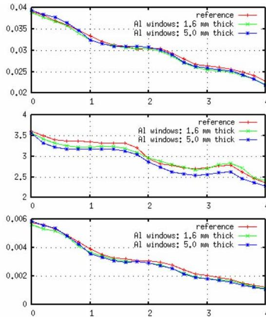
Figure 5: Cooling performance. Shown are the results of simulations (including the effects of windows) of the transverse (top), longitudinal (middle) and 6D (bottom) emittances in the 6DMANX HCC. The axes are emittance (m rad) vs. length of cooling channel (m).
